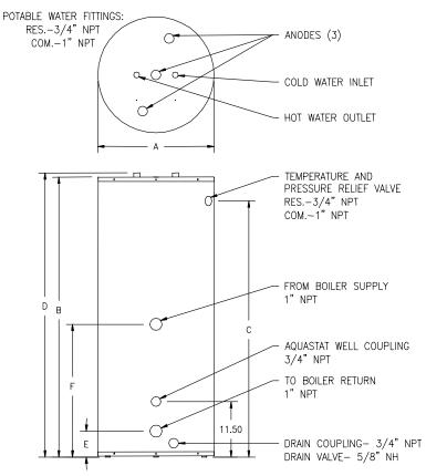
Figure 1 – Tank Layout
