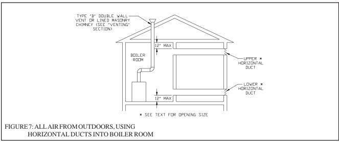
• The "free area" of an opening takes into account the blocking effect of mesh, grills, and louvers. Where screens are used, they must be no finer than  $\frac{1}{4}$ " (4 x 4) mesh.
