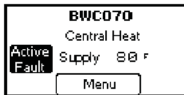
Figure 11.0c: Home Screen with Active Fault
