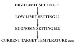
The display will return to boiler temperature (default) if Test/Settings Button in not pressed for 5 seconds.
