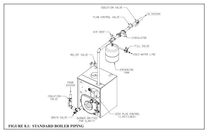
1) Relief valve (Required) - Mount the relief valve on the top left side of the boiler as shown in Figure 8.1 using the 3/4" nipple provided. The relief valve shipped with the boiler is set to open at 30 psi. This valve may be replaced with one having a pressure up to the "Maximum Allowable Working Pressure" shown on the rating plate. If the valve is replaced, the replacement must have a relief capacity in excess of the DOE heating capacity for the boiler.
