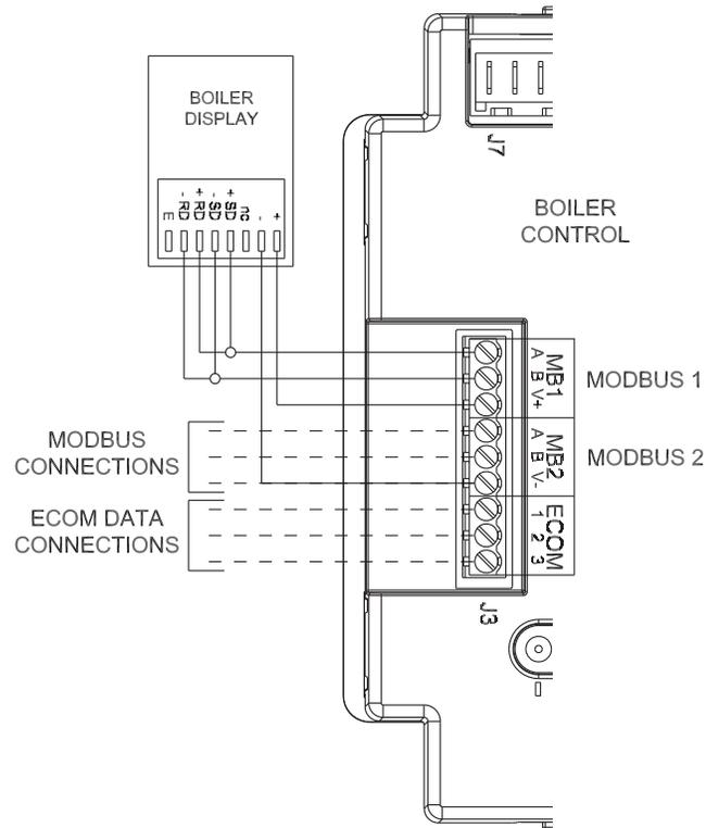
**Figure 11.6: J3 Field Wiring**
