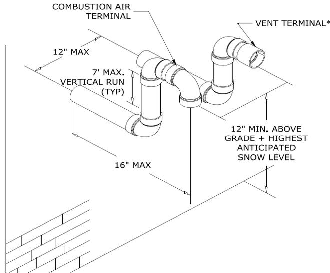
**Figure 7.12: Snorkel Terminal Configuration (CPVC/PVC Vent Systems Only)**
