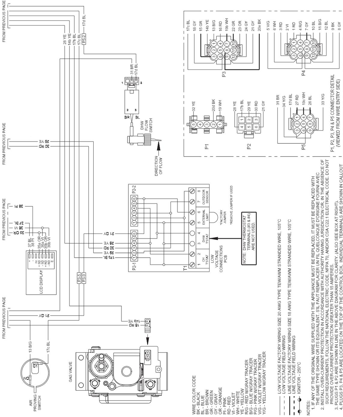
Figure 11.8: Internal Wiring Connections Diagram
