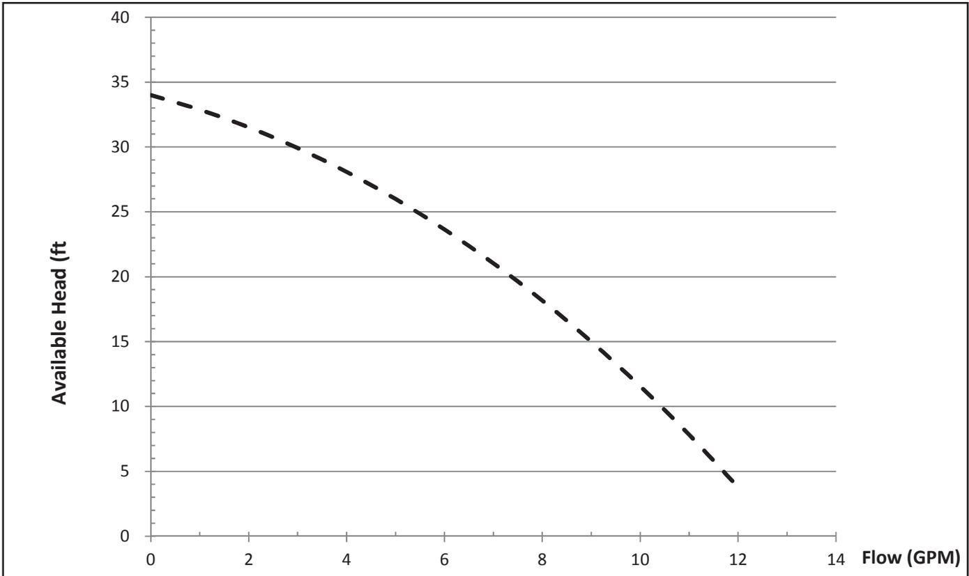
**Figure 9.7b: 150/180 Net Circulator Curve (Taco 0013)**
