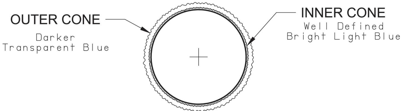
**Figure 12.3: Burner Flame**
