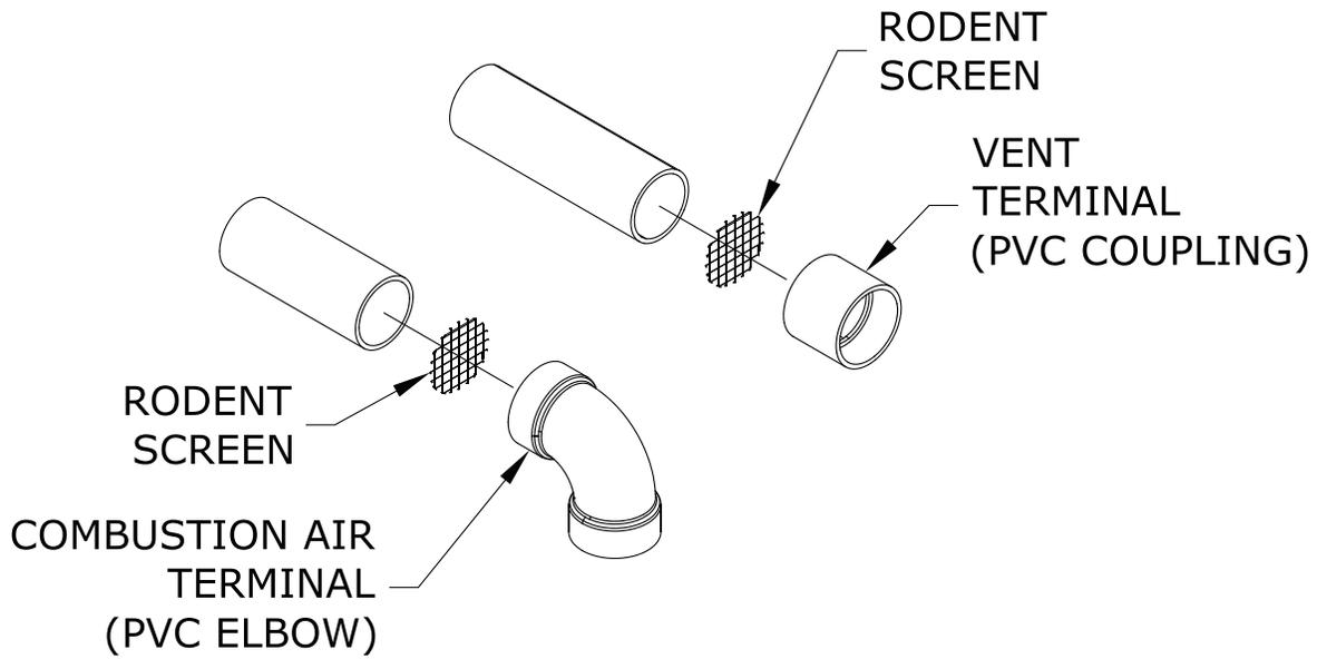
**Figure 7.28: Installation of Standard Horizontal Terminals**
