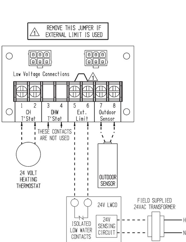
**Figure 11.4b: 24 Volt LWCO Field Wiring Using 24 VAC Transformer**
