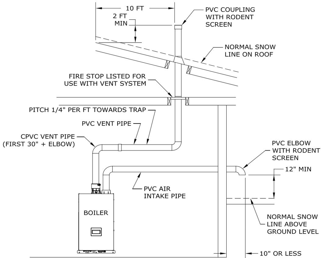
**Figure 7.22: Split Rigid Vent System (Vent Options 11-14)**
