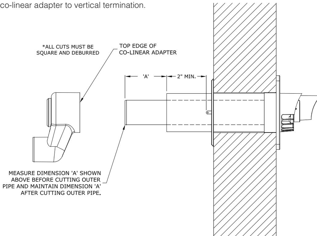
**Figure 7.38: Cutting DuraVent PolyPro Horizontal Concentric Vent Terminal**
