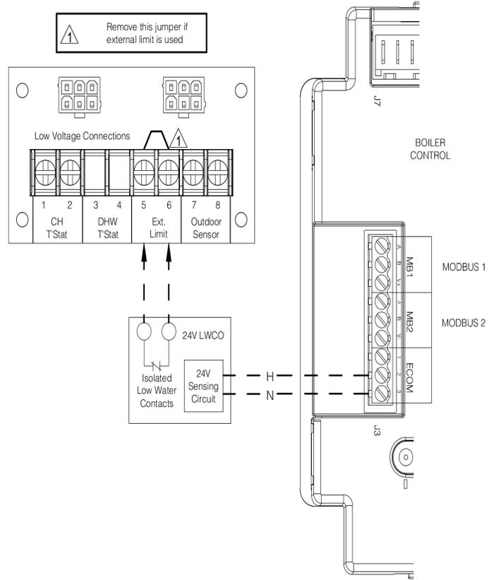
**Figure 11.4c: 24 Volt LWCO Field Wiring Using Control ECOM**
