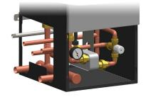
Phantom® Combi-Kit Add domestic hot water capabilities directly to the Phantom® 150 and 180 with one easy step, precisely matching to the existing boiler connections. The kit includes mixing valve, plate heat exchanger and the EZ-Loop Low Loss Header.
