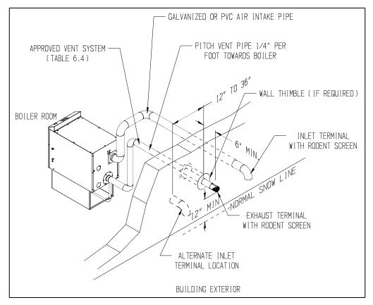
FIGURE 6.2: HORIZONTAL TWIN PIPE VENTING (VENT OPTIONS 1,2,3)
