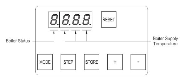
Figure 11.1: Normal Display In Standby Mode
