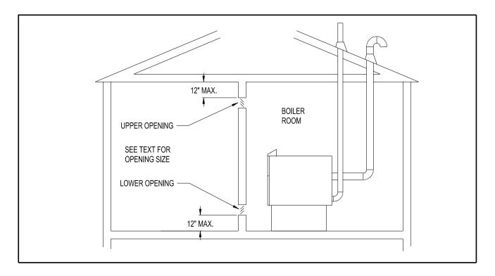
Figure 5.1: Boiler Installed In A Confined Space, Ventilation Air From Inside
