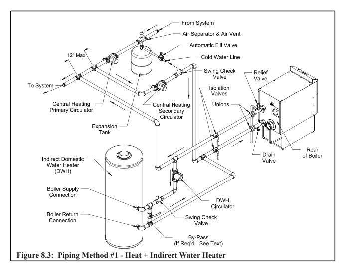
Feet Straight Pipe. From Table 8.7, we see that a Taco 008 will pump at 8 GPM through a BWC300 with 56 equivalent feet and an MS-40. The Taco 008 is just large enough to work in this application (a Taco 009 could also be used if desired).
