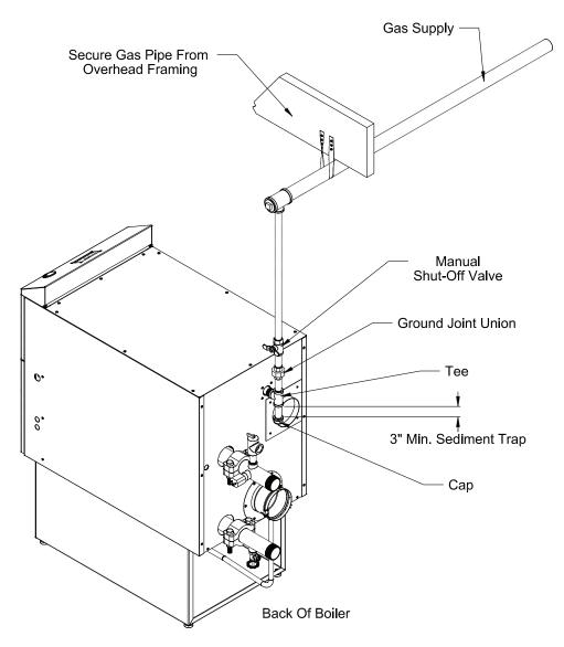
Figure 7.1: Gas Connection To Boiler
