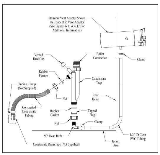
FIGURE 6.23: CONDENSATE PIPING ARRANGEMENT
