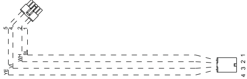
Inner Vestibule Blower Control Harness
