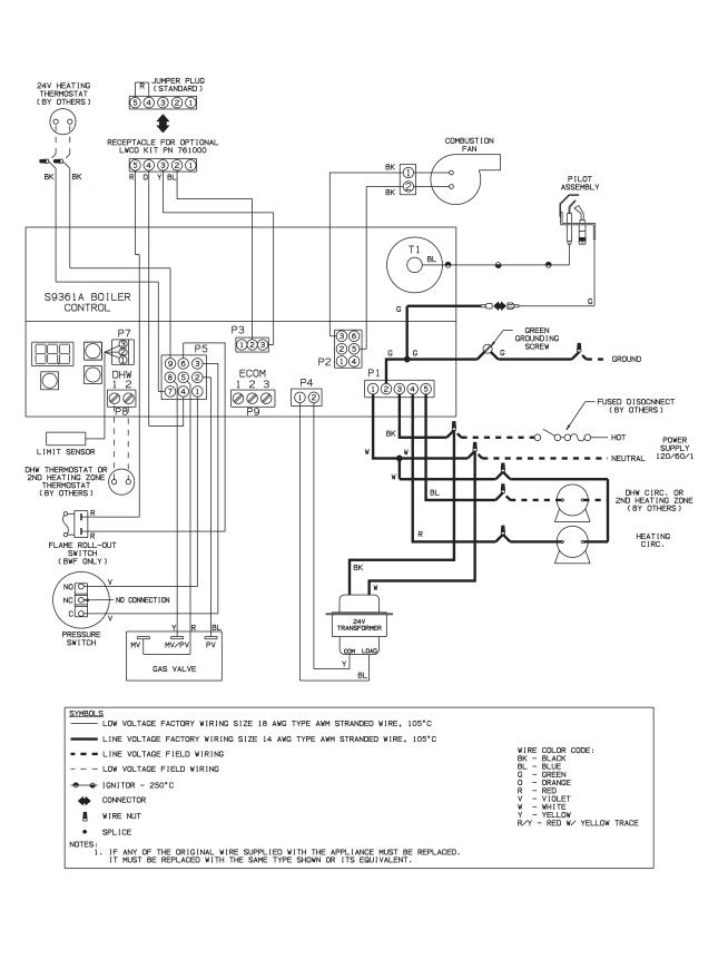
FIGURE 9.2: INTERNAL CONNECTIONS DIAGRAM
