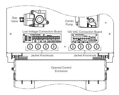
Figure 13-1: Location 120 VAC and Low Voltage Connection Boards
