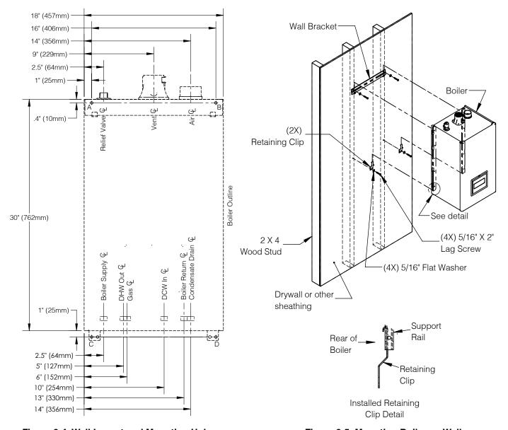
Figure 6-4: Wall Layout and Mounting Holes
