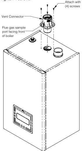
Figure 6-2: Installing Vent Connector
