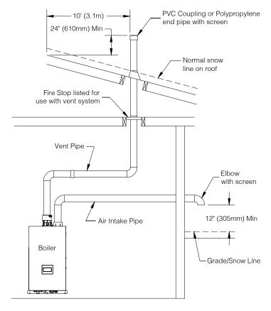
Figure 9-5: Alternate Vertical Vent/Sidewall Air Terminal
