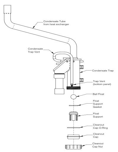
**NOTICE:** Attempting to clean heat exchanger or trap with anything other than water or vinegar could damage heat exchanger or result in condensate backup, causing boiler to shut down.
