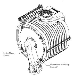
Figure 18-1: Ignitor/Flame Sensor Location
