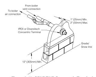
Figure 8-10: CPVC/PVC Concentric Terminal
