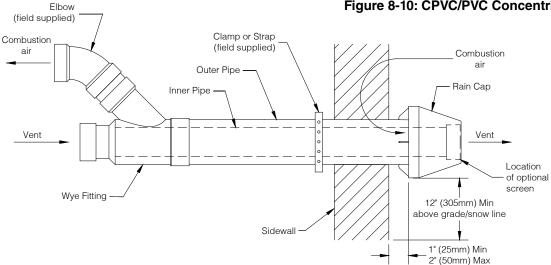
Figure 8-11: CPVC/PVC Concentric Terminal Installation
