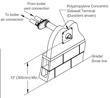
Figure 8-14: Polypropylene Concentric Terminal
