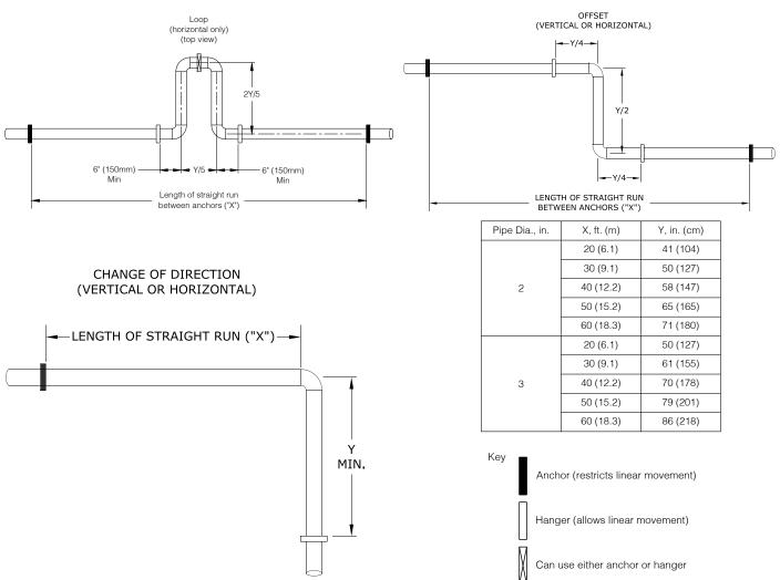
Figure 7-15: CPVC/PVC Venting Expansion Loops
