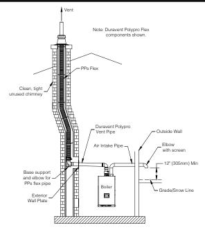
Figure 9-16: Masonry Chimney Chase System
