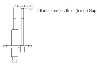
Figure 18-2: Ignitor/Flame Sensor Spark Gap
