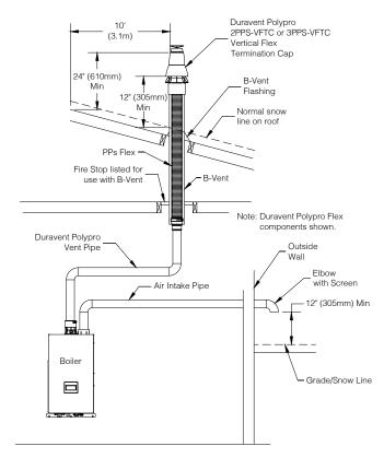
Figure 9-14: Polypropylene B-vent Chase with Sidewall Air Terminal
