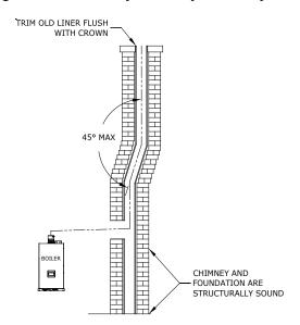
Figure 9-17: Masonry Chimney Chase Requirements
