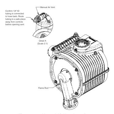
Figure 15-1: Manual Air Vent Location
