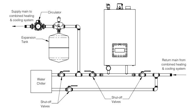
Figure A-1: Isolated Boiler from Refrigeration System
