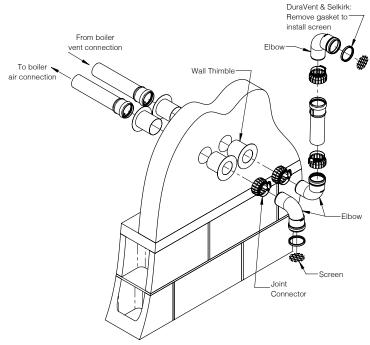
Figure 8-6: Polypropylene Fittings Terminal Assembly
