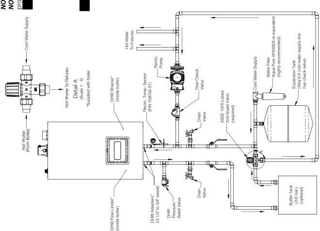
Figure 11-3: DHW Piping with Recirculation
