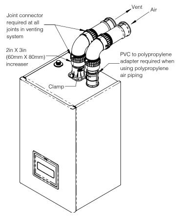
Figure 7-19: Near Boiler Polypropylene Venting with Increaser
