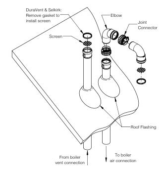
Figure 9-4: Polypropylene Fittings Terminal Assembly
