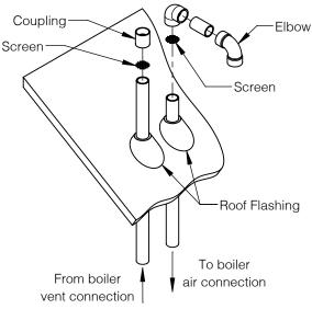
Figure 9-3: CPVC/PVC Fittings Terminal Assembly
