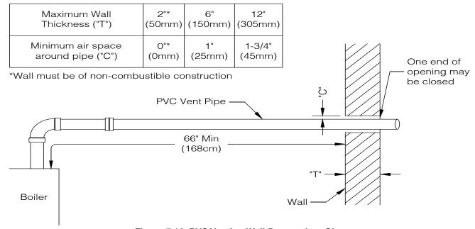
Figure 7-14: PVC Venting Wall Penetration Clearance
