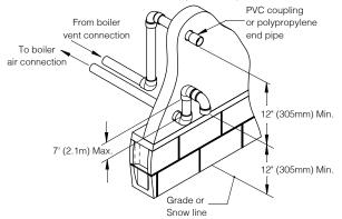
**Figure 8-4: Alternate Fittings Terminal**
