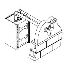
Figure 7-1: Sidewall Termination with Fittings see Section 8 for details
