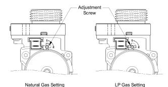
Figure 15-3: Gas Valve Fuel Setting
