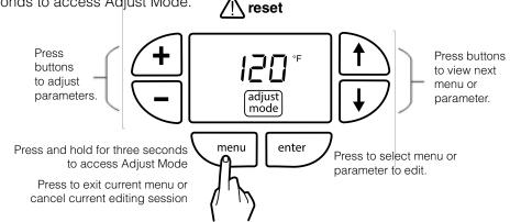
Figure 16-7: Adjusting Parameters
