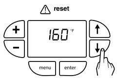
Figure 16-3: Viewing Boiler Status
