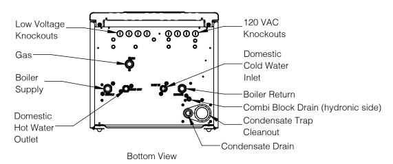
Figure 3-7: Boiler Connections
