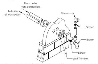
Figure 8-5: CPVC/PVC Fittings Terminal Assembly
