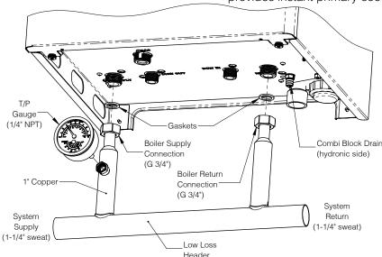
Figure 10-1: Low Loss Header Connections
