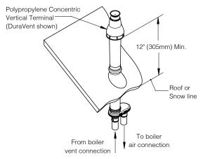
Figure 9-10: Polypropylene Concentric Terminal
