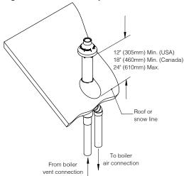
Figure 9-6: CPVC/PVC Concentric Terminal
