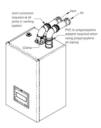
Figure 7-18: Near Boiler Polypropylene Venting
