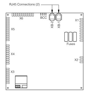
Figure 13-4: Boiler-to-Boiler Connections
