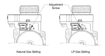
Figure 6-3: Gas Valve Fuel Setting
