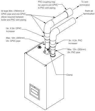
Figure 7-13: Near Boiler CPVC/PVC Venting with Increaser
