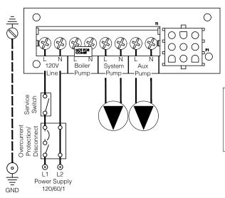
Figure 13-2: 120 VAC Connections
