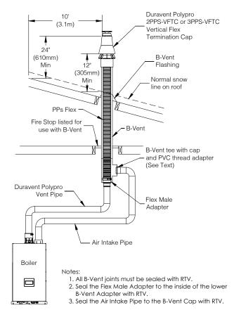
Figure 9-12: DuraVent Polypropylene B-vent Air Chase System
