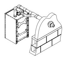
Figure 7-3: Sidewall Concentric Termination see Section 8 for details
