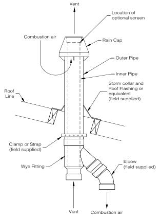
Figure 9-7: CPVC/PVC Concentric Vertical Installation
