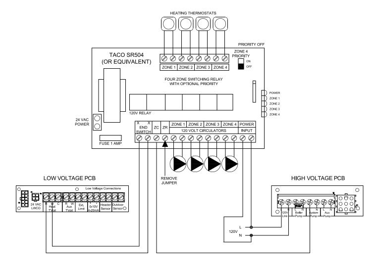
\*\*\*USE SAME POWER SOURCE FOR ALL CONTROLS AND ENSURE POLARITY TO ALL CONTROL DEVICES IS CORRECT
