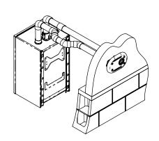
Figure 7-2: Sidewall Low Profile Termination - see Section 8 for details
