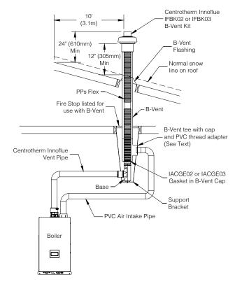
Figure 9-13: Centrotherm Polypropylene B-vent Air Chase System
