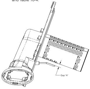
Figure 18-3: Ignitor/Flame Sensor to Burner Gap
