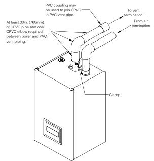
Figure 7-12: Near Boiler CPVC/PVC Venting
