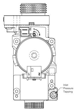
Figure 15-9: Gas Valve Inlet Pressure Tap
