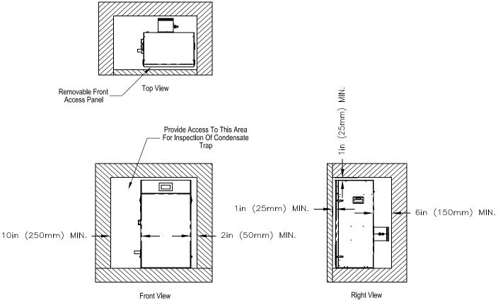
Figure 3-3: Clearances To Combustible and Non-combustible Material
