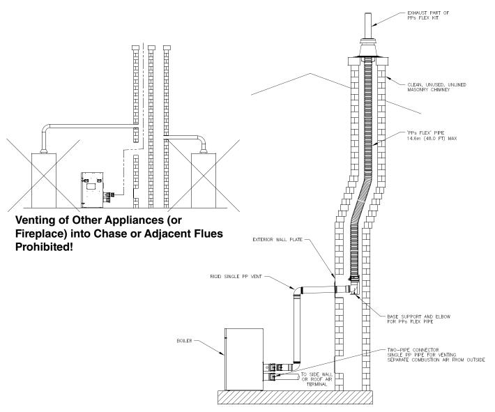
Figure 4-29: Flexible Vent in Masonry Chimney with Separate Combustion Air Intake
