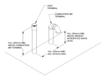
Figure 4-9: Direct Vent - Vertical Terminations
