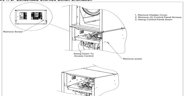
Figure 11-3: Control Compartment Access for Stacked Boiler Installations
