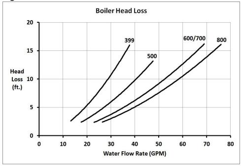
Figure 6-7: Boiler Head Loss
