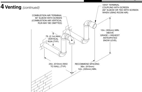
Figure 4-7: Direct Vent - Sidewall Snorkel Terminations
