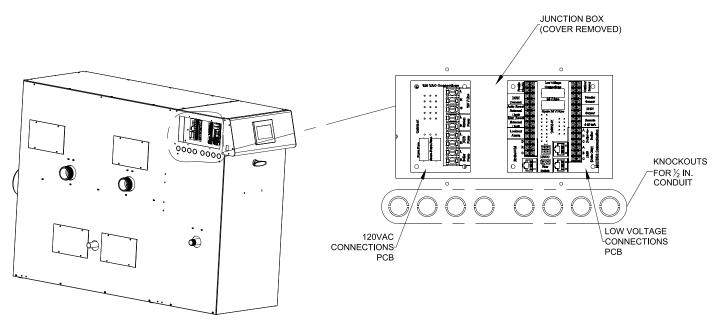
Figure 8-2: PCB Locations for Field Wiring
