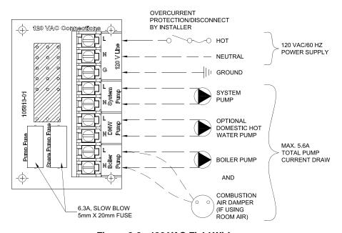
Figure 8-3: 120 VAC Field Wiring
