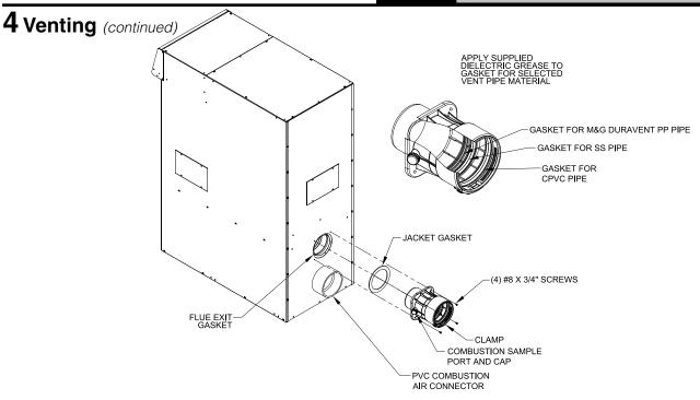
Figure 4-15: Field Installation CPVC/PP/SS Vent Connector
