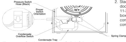
Figure 11-2: Condensate Overflow Switch Orientation
