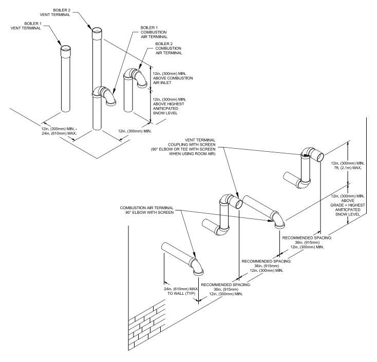
Figure 4-34: Multiple Boiler Direct Vent Termination
