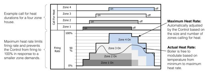
Figure 10-10: Four Zone House (with Zone Control Connected)
