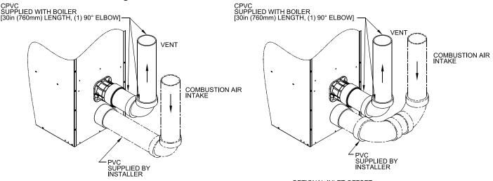
Figure 4-16: Near-Boiler Vent/Combustion Air Piping
