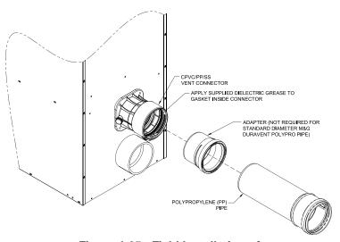
Figure 4-25: Field Installation of Polypropylene Vent Adapter
