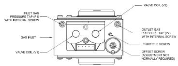
Figure 9-5: Gas Valve Detail
