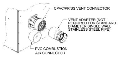
Figure 4-33: Field Installation of Stainless Steel Vent Adapter
