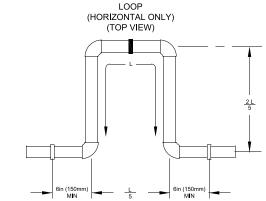
Figure 4-17: CPVC/PVC Expansion Loop and Offset
