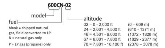
Figure 10-9: Selecting Boiler Type
