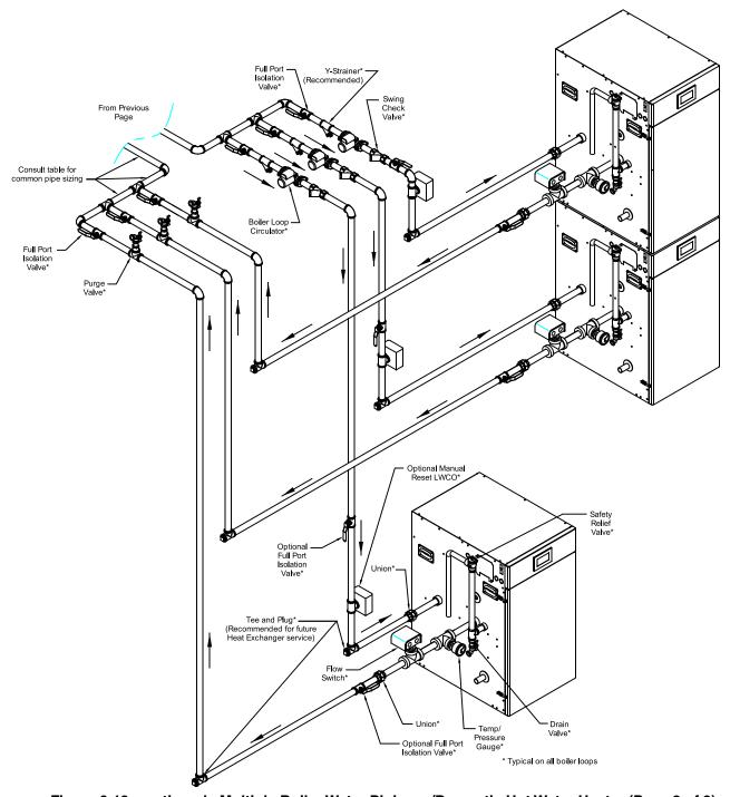
Figure 6-16, continued: Multiple Boiler Water Piping w/Domestic Hot Water Heater (Page 2 of 2)
