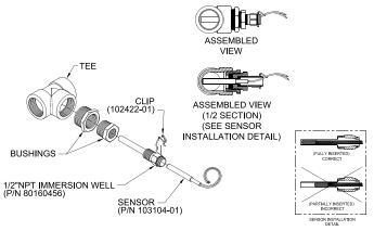
Figure 6-15: Alternate "Immersion" Type Header Sensor or DHW Heat Source Sensor Installation Detail
