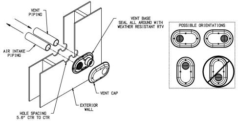
Figure 4-8: Direct Vent - Sidewall Low Profile Termination
