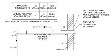
Figure 4-18: Wall Penetration Clearances for PVC Vent Pipe
