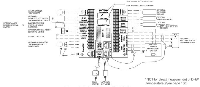
Figure 8-4: Low Voltage Field Wiring
