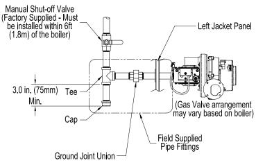
Figure 7-5: Recommended Gas Piping
