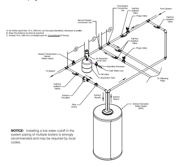
Figure 6-16: Multiple Boiler Water Piping w/Domestic Hot Water Heater (Page 1 of 2)
