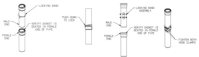
Figure 4-27: Locking Band Clamp Installation, M&G DuraVent or Centrotherm InnoFlue
