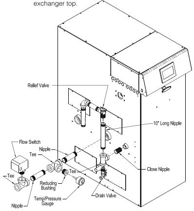
Figure 6-1: Factory Supplied Piping and Trim Installation - PHNTM399C
