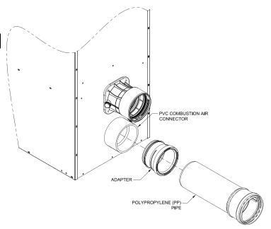
Figure 4-26: Field Installation of Polypropylene Combustion Air Adapter
