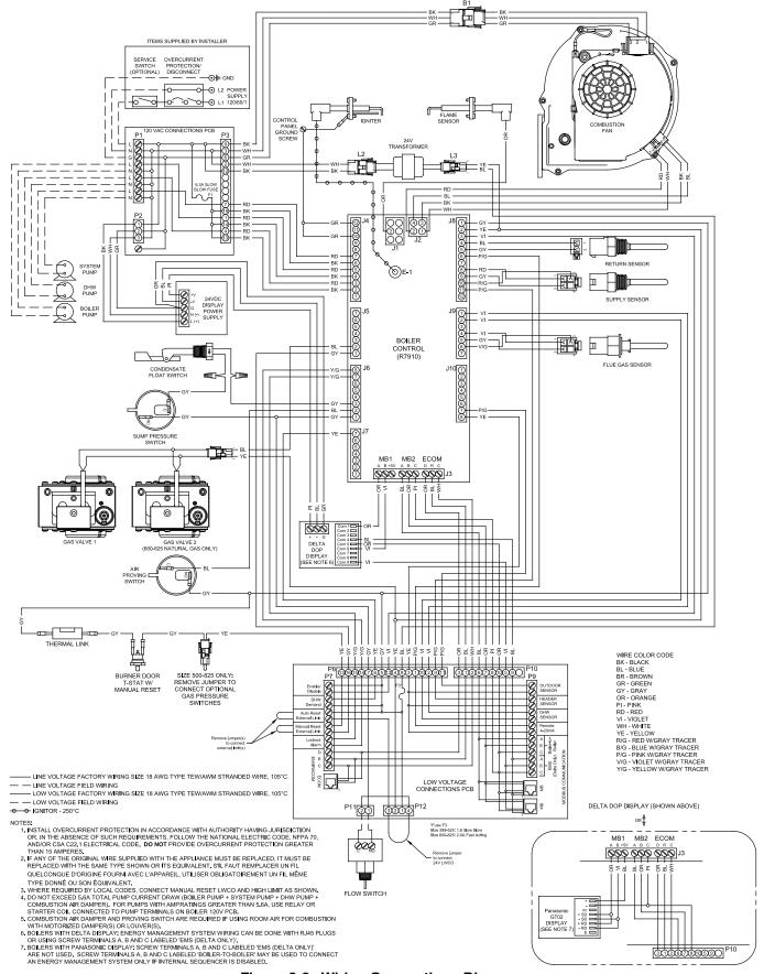
Figure 8-6: Wiring Connections Diagram
