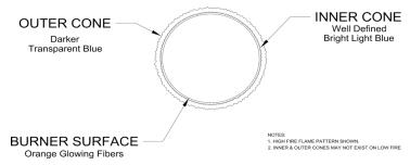
Figure 9-4: Burner Flame
