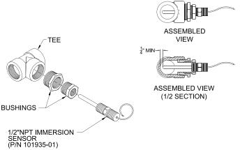
Figure 6-14: Recommended Direct Immersion Header Sensor or DHW Heat Source Sensor Installation Detail
