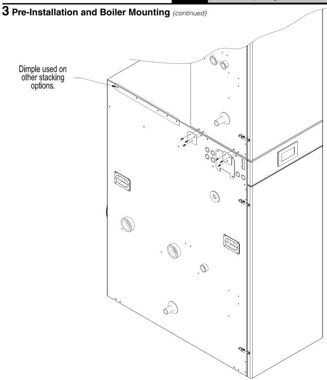
Figure 3-5: Boiler Stacking
