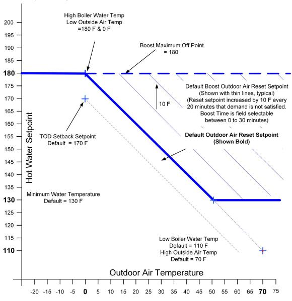
Figure 10-12: Outdoor Reset Curve - Typical for Central Heat and Auxiliary Heat
