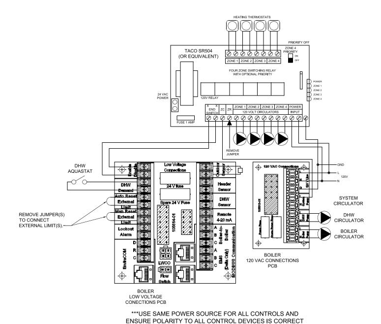
Figure 8-7: Modified Wiring For DHW Priority When Using Low Flow Circulator Piped Off System Header - Heating (with Central Heating Circulators) Plus Alternately Piped Indirect Water Heater
