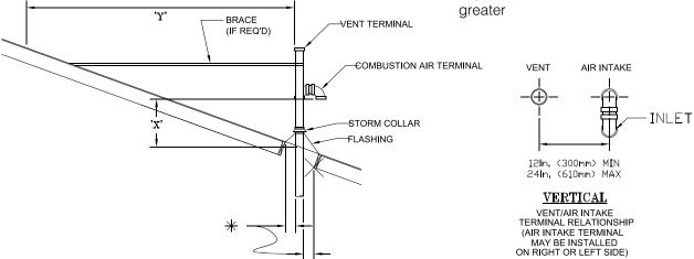
\*\* VENT PIPE MINIMUM CLEARANCE TO COMBUSTIBLE MATERIAL IS 1in. (25mm). COMBUSTION AIR PIPE MINIMUM CLEARANCE TO COMBUSTIBLE MATERIAL IS 75RO
