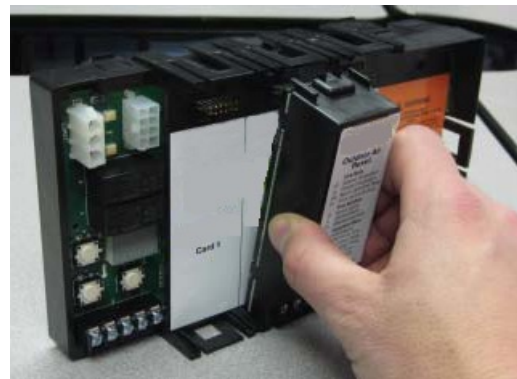
Insert OC Panel High Limit Aquastat Card into selected slot
